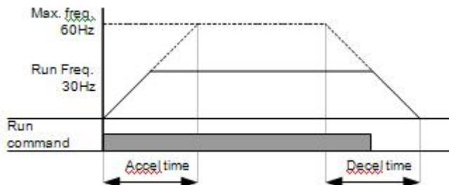
More precise time unit can be set corresponding to load characteristics as shown below
